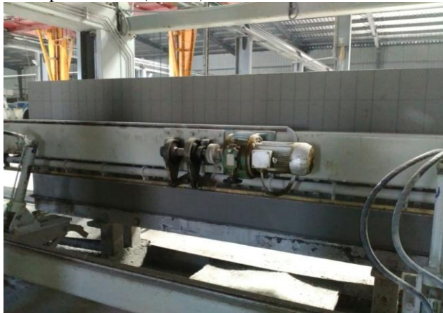
Fig.4 wire cutting of fresh mixture of AAC block
