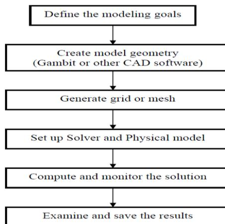
**Figure 4.1:** Steps involved in the CFD analysis procedure
