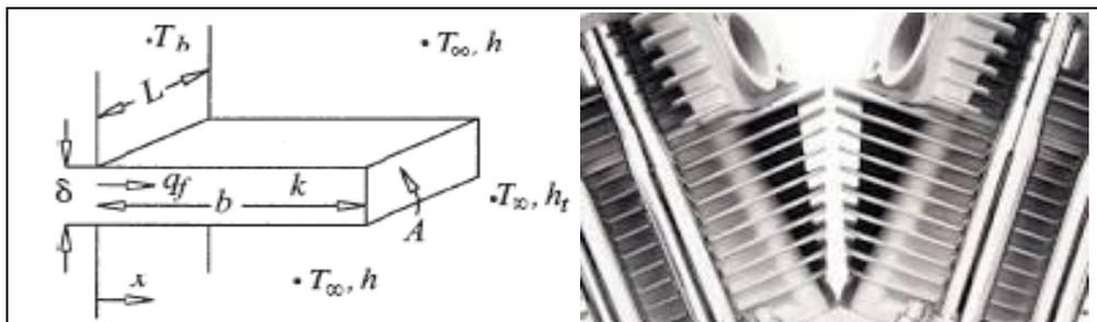
**Figure 3.3:** Structure of fins
